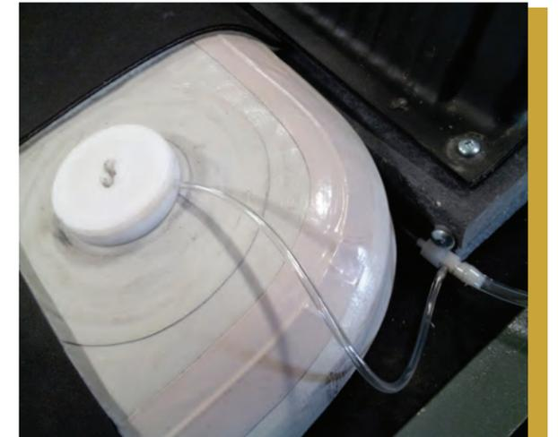
Air tubes connecting a row of mats remain connected to a regulator and air tank, so adding a little air when required couldn't be easier.
