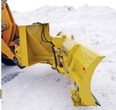
Our mounts allow for one-person, tool-less quick attachment to Degelman's 3500 and 5700 series bulldozer blades. These blades are doublewalled, non-ribbed and built to last. Depending on what projects you decide to tackle, we've got several blade and width choices:
