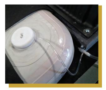
Air tubes connecting a row of mats remain connected to a regulator and air tank, so adding a little air when required couldn't be easier.
